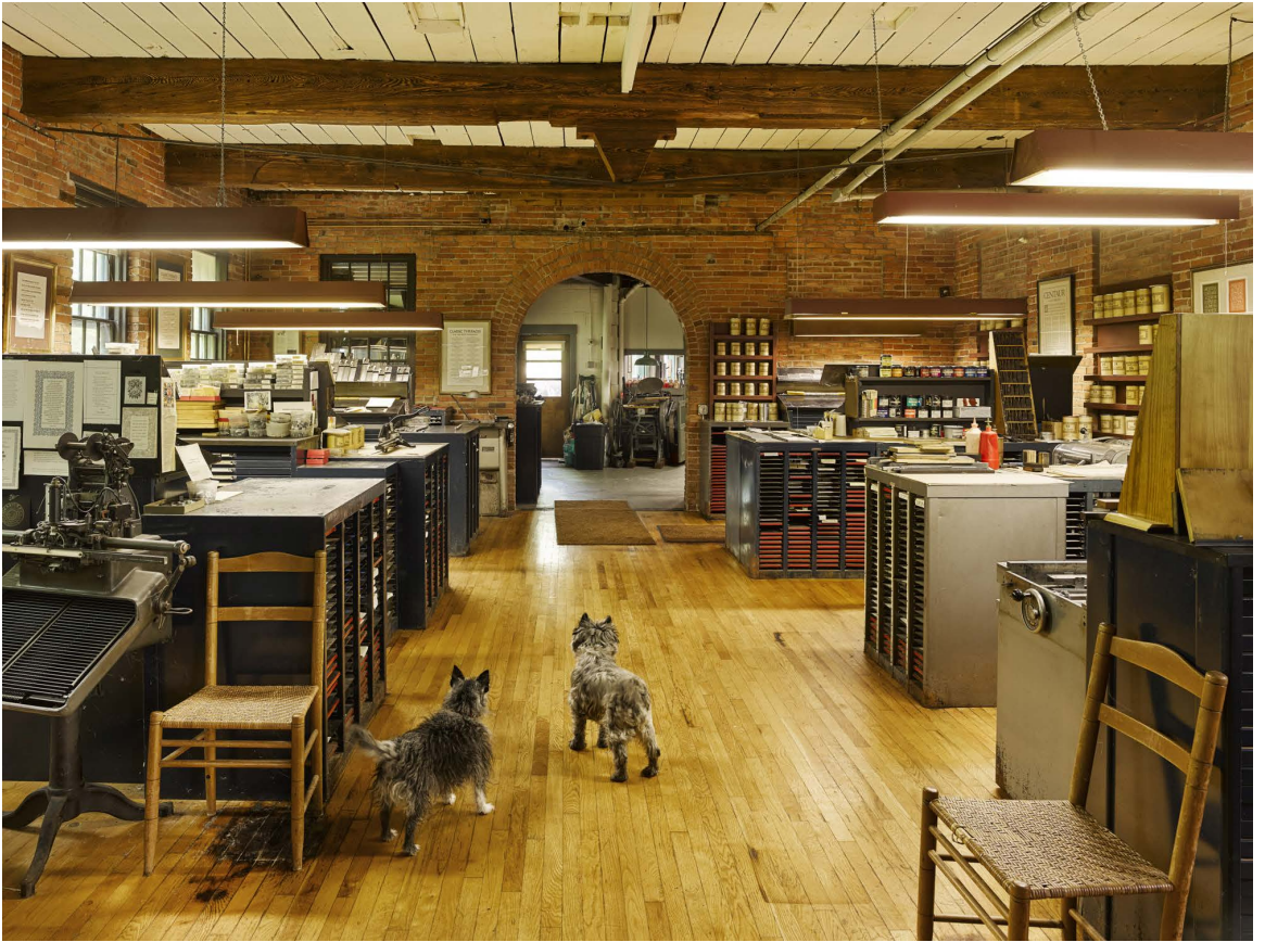
7. The composing room with Monotype keyboards, Vandercook proof presses, galley cabinets, 700 cases of Bixler-cast type, and two dogs.
