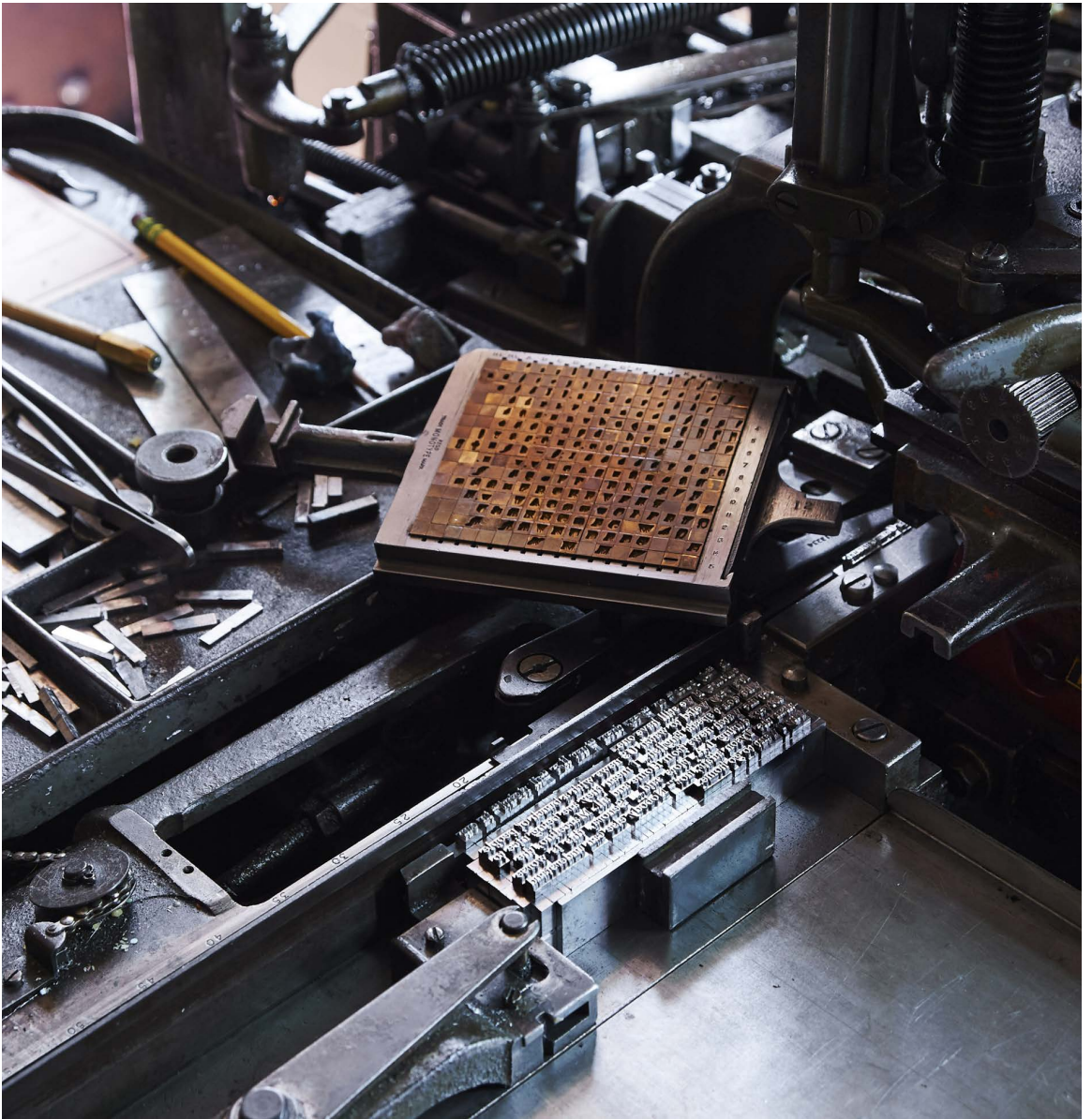
6. A Monotype mat case removed from the caster, containing 255 matrix character positions, capable of carrying letters from 8- to 14-pt., providing the simultaneous use of Roman, Italic, and Small Cap alphabets.
