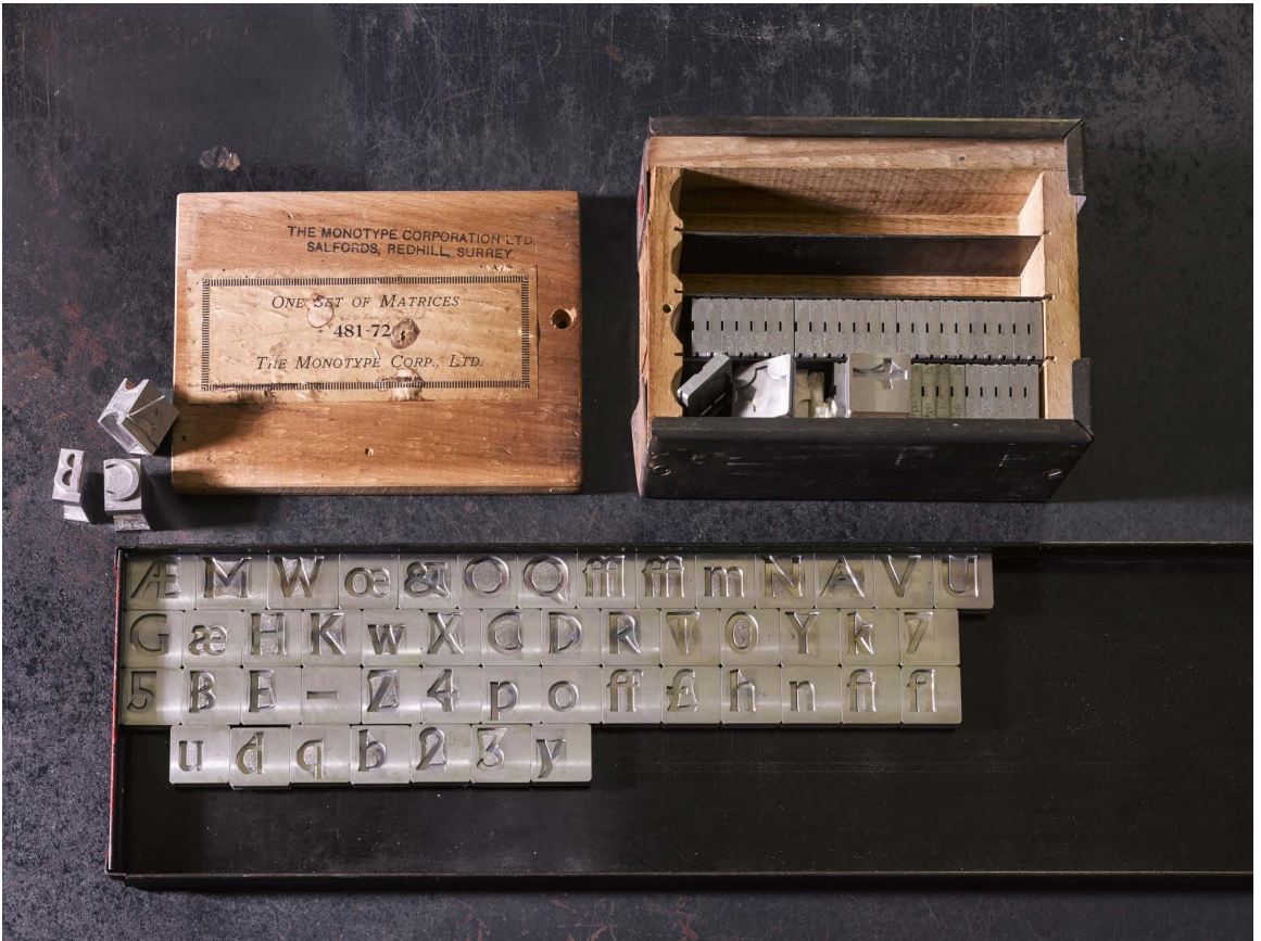
8. English Monotype display mats for 72-pt. Albertus. Each matrix can cast an unlimited number of types from the Supercaster.
